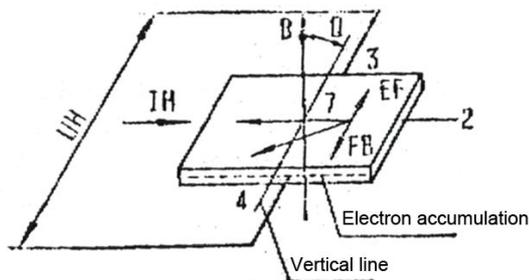
current is given, at this time, the Hall electric potential  $V_H$  will be in direct ratio to tested magnetic field  $B$ . if the position of Hall device and magnetic field is fixed up, when angle  $\theta=0$ (that is the outputs comes to max.),  $V_H$  is in direct ratio to  $B$ .
