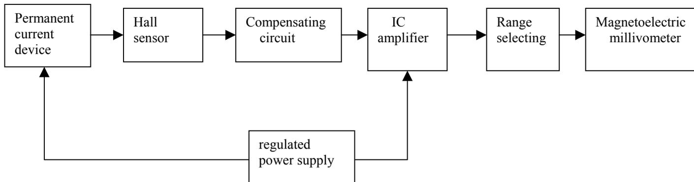
1. Hall sensor: the apparatus has one CT5A-1 Hall sensor and can test transverse magnetic field. Also it installs gallium arsenide Hall device and the dimension of CMOS chip is  $1 \times 1 \times 0.2 \text{mm}^3$ , the device is glued on the insulated scaleboard and protected by flat copper shell outside. When it installs testing hand, the figure size of sensor is  $3.2 \times 1.1 \times 35 \text{mm}^3$ , the device is coordinately installed the head of copper tube. (Ref. to drawing 2)
