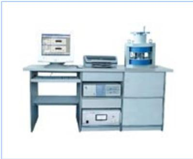
Automatic measurement on hysteresis loop and demagnetization curve of permanent-magnet material, accurate measurement on magnetic characteristic parameters such as remanence  $B_r$ , coercive force  $H_cB$ , intrinsic coercive force  $H_cJ$  and maximum magnetic energy product  $(BH)_{max}$ .
