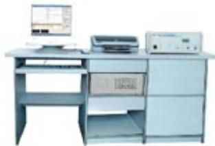
Automatic measurement on basic magnetization curve and magnetic hysteresis loop under static state of soft magnetic material, accurate measurement on static magnetic characteristic parameters such as initial permeability  $\mu_i$ , maximum permeability  $\mu_m$ , saturation magnetic induction  $B_s$ , remanence  $B_r$ , coercive  $H_c$  and hysteresis losses  $P_u$ .
