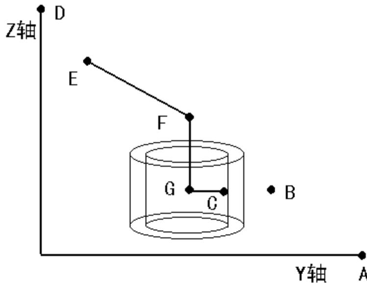
Explanation: The drawing shows the physical position of parameters in inner ring surface test. E.g, a magnet with size of id=8mm. Set the pulse value of returning point in Z axis as 6600, pending testing point 2000, while pulse value in Z axis 7700, 2350 pulse in Y axis. A is the zero point of Y axis, B is pending testing position (350), C is
