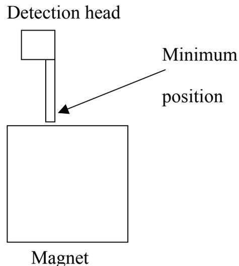
between detection head and magnets to protect the equipment.
